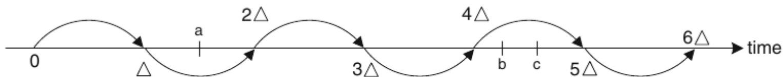
Fig. 1.3 Clock advancement in a time-driven simulation
