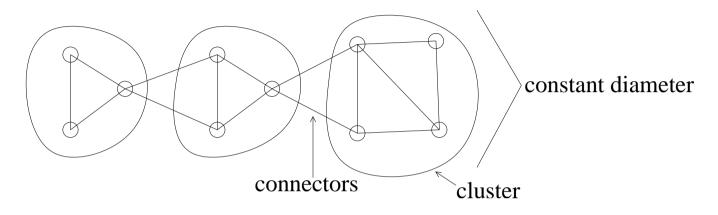
clusters: partiton of V(G) into disjoint sets  $V_1, \ldots, V_k$ each  $G[V_i]$  is connected and has constant diameter
